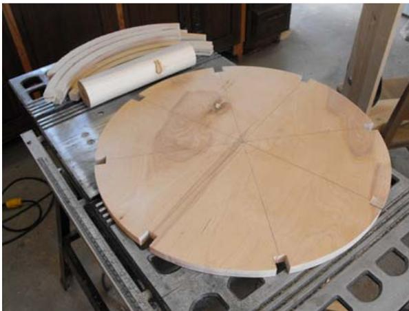
Assembly of the components was then done with the addition of the nose rope loop to complete the frame.
