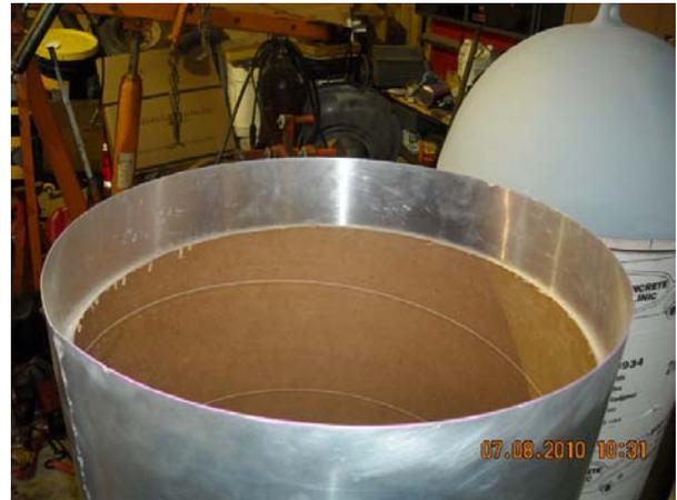
Aluminum fitted to concrete forms the tube, welded and filled to cover any gaps.
