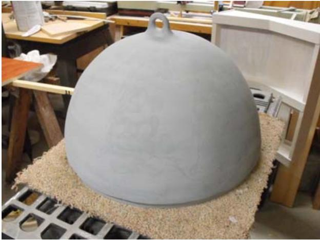
Mounting plate was attached – note ¼ inch lip on the bottom. The mounting plate is to go inside the body of the torpedo and the warhead matches the diameter of the torpedo.
