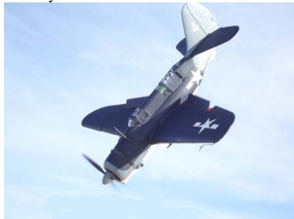
The SB2C Helldiver was a replacement for its predecessor, the Douglas Dauntless (SBD). The model is mounted in the diving position, with dive flaps open – all dive flap perforations have been drilled out.
