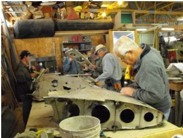
Mike Hudak and other Sq.4 members working on a Horizontal Stab.
