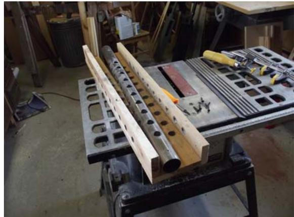
Cooling jacket with holes drilled out –
